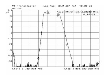
The above picture shows the GPS35 frequency response from 300 kHz to 3 GHz. Ultimate rejection is typically  $> 80~\mathrm{dB}$
